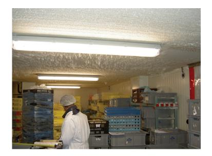
streams into the -20°C store every time the doors are opened, due to the frequent deliveries throughout the day. The result is frosting and icing up of the floors inside and outside the storage area, icing of refrigeration components, such as the evaporator, and also frosting of product making it difficult for the food technicians to read the product labels.
